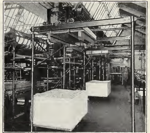
Rouse Paper Lift in Plant of Max Lau Colortype Co., Chicago Nearly 600 in use.
